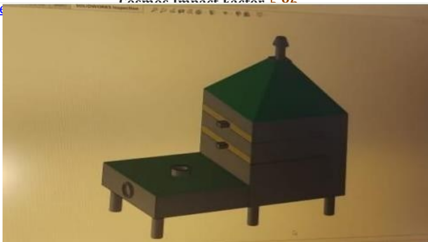
Fig. 3D Cad Model of solar vegetable dryer
